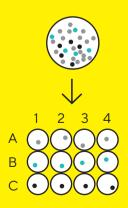
In order to analyze or cultivate single cells, the CellCelector Flex deposits each picked object in one well.
