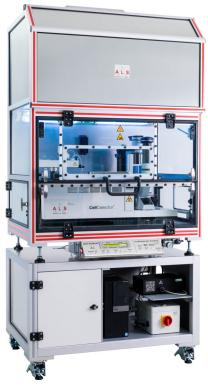
ALS CellCelector installed in ALS FlowBox™ Incubator with temperature, humidity and CO<sub>2</sub> control. The system can be also placed within a standard biosafety cabinet.
