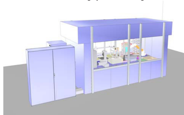
Fig. 2. Machine enclosure with laminar flow (right), external control system (left) and external incubator (left back)
