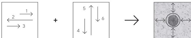
For picking of adherent colonies the CellCelector Flex combines a very gentle, crosswise scrape movement with a simultaneous aspiration of the colony. This gently loosens the colony from the base of the culture plate or feeder cell layer.
