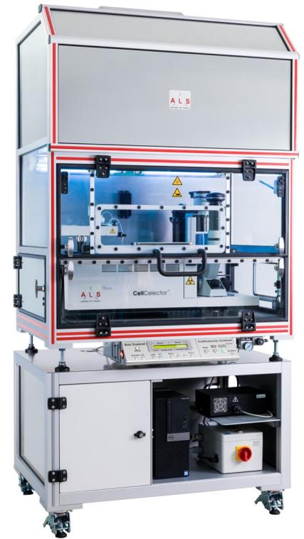
ALS CellCelector installed in ALS FlowBox™ Incubator with temperature, humidity and CO<sub>2</sub> control. The system can be also placed within a standard biosafety cabinet.
